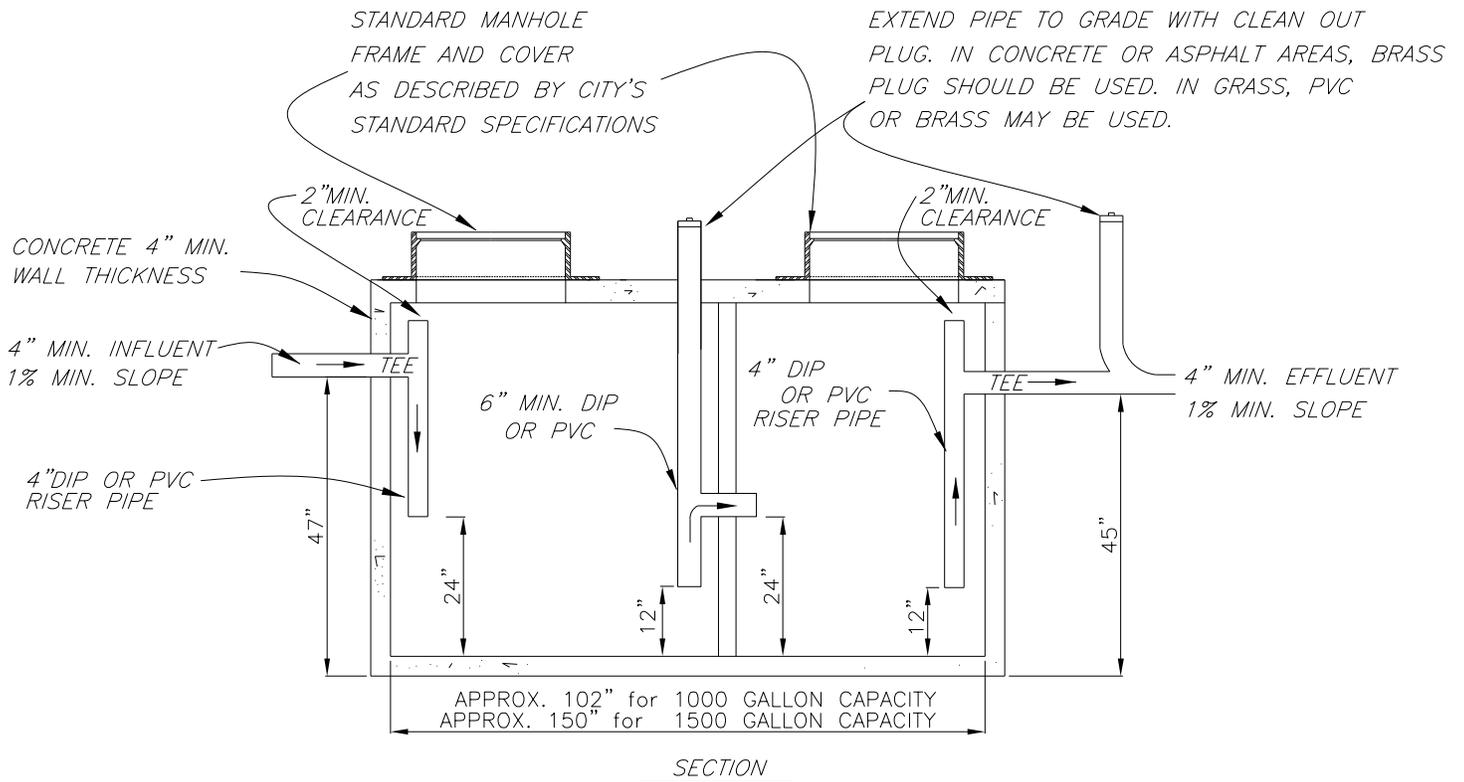
1. THE INVERT OF THE INLET PIPE SHALL NOT BE LESS THAN 2" ABOVE THE INVERT OF THE OUTLET PIPE.
